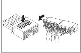
Push the terminal retainer down to the temporary lock position.
