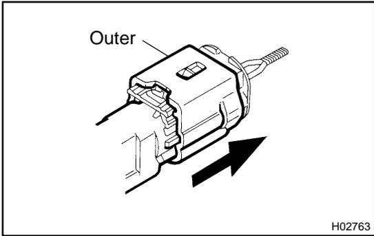
**4. DISCONNECTION OF AIRBAG FRONT SENSOR AND SIDE AIRBAG SENSOR CONNECTOR**
