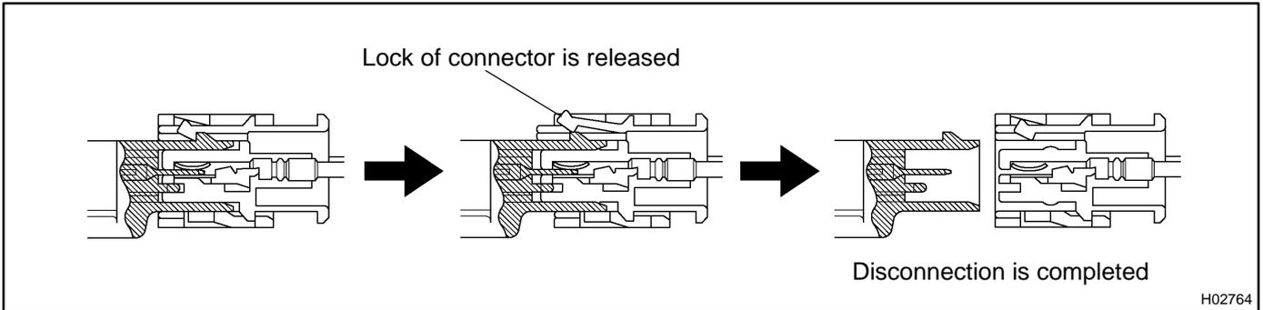
**5. CONNECTION OF CONNECTORS FOR AIRBAG FRONT SENSOR AND SIDE AIRBAG SENSOR**
