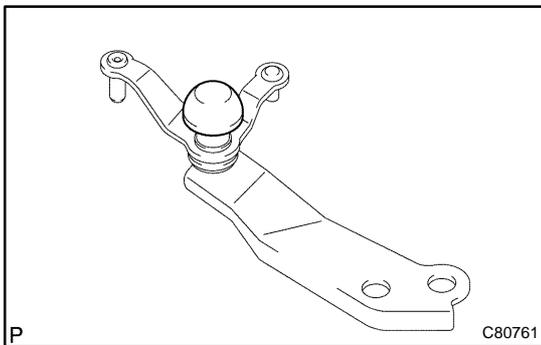
**2. REMOVE SELECTING BELLCRANK DUST COVER NO.1**
