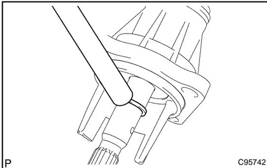
**11. REMOVE CONTROL SHAFT COVER OIL SEAL**
