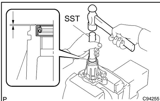
**12. INSTALL CONTROL SHAFT COVER OIL SEAL**
