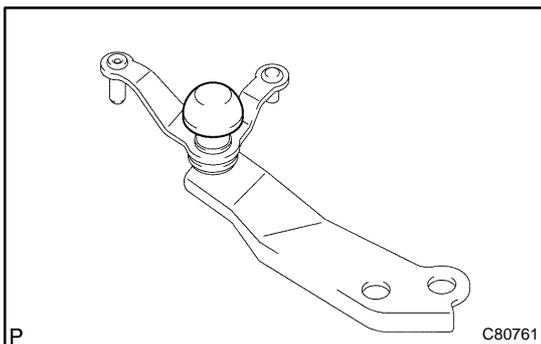
**21. INSTALL SELECTING BELLCRANK DUST COVER NO.1**
