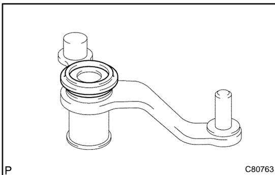
**4. REMOVE SELECTING BELLCRANK DUST COVER NO.2**
