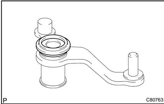
**19. INSTALL SELECTING BELLCRANK DUST COVER NO.2**
