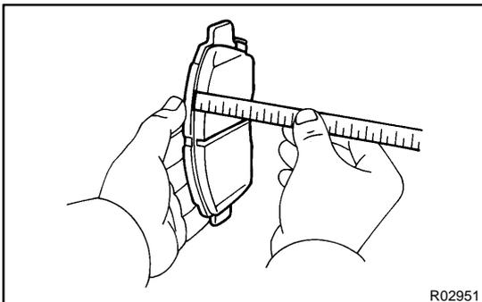
**14. INSPECT PAD LINING THICKNESS**
