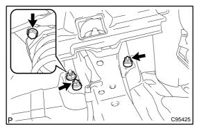
(b) Remove the 2 nuts and bolt.
