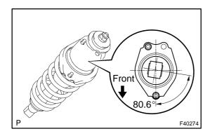
(e) Position the rear spring front bracket sub–assy LH with rear coil spring insulator upper LH as shown in the illustration.
