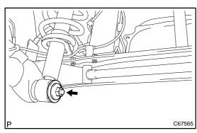
(c) Remove the nut, rear shock absorber LH cushion retainer and rear shock absorber with coil spring.
